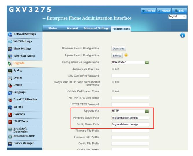
Figure 17: GXV3275 Upgrade Configuration via Web GUI
