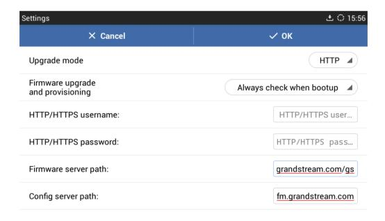
Figure 16: GXV3275 Upgrade Configuration via LCD
